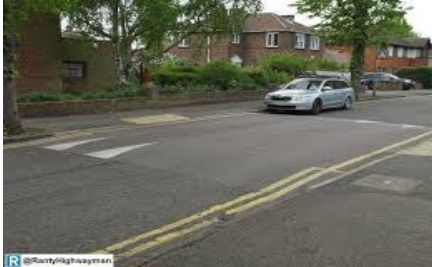
A Speed Table Cost per feature = £2,400 (approx) -----
